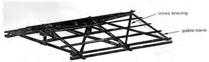
Figure-4b: Earthquake bands and reinforcement (Pitched Roof for E.Q).
