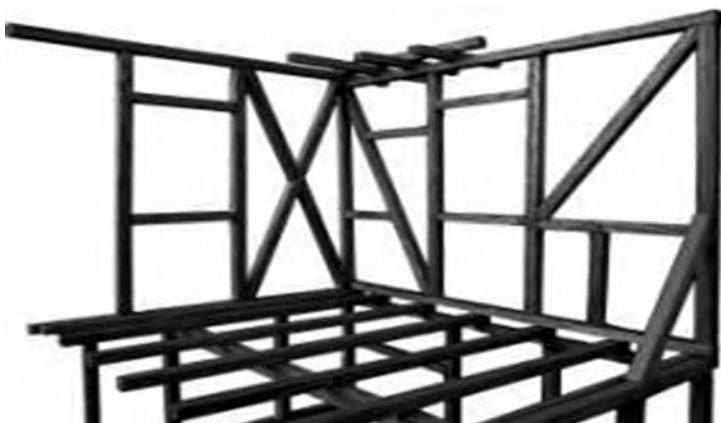
Figure-4: Dhajji-Diwari System: Timber frame with infill walls.
